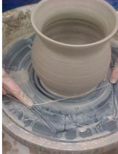
Remove the bat from the wheelhead. You will probably have to use a slim blade of some kind to break the suction of the slip. Put the pot aside, but don't let it dry out completely. When it is leather hard, it will need to be trimmed.
