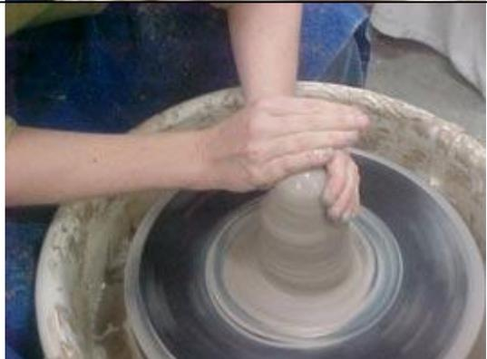
To move downward with the clay, both hands must supply force. Remember to brace your elbows! The right hand supplies downward pressure (like a continuous karate chop). The left hand moves out horizontally (from 6 o'clock to 12 o'clock on the wheelhead). You've got that clay locked in a moving vice grip.
