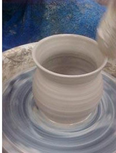
Be sure to take as much clay as you can off the bottom of the pot near the wheelhead. This saves you trimming work later. You can use a sponge and/or a wooden knife or rib.
